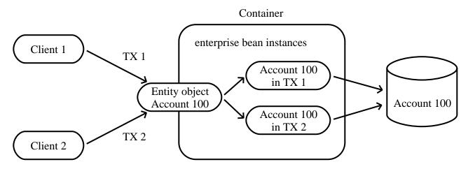
Figure 13. Multiple Clients Can Access the Same Entity Object Using Multiple Instances
