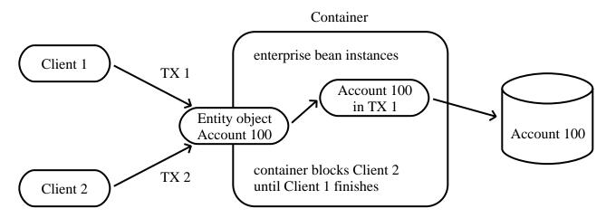
Figure 8. Multiple Clients Can Access the Same Entity Object Using Single Instance
