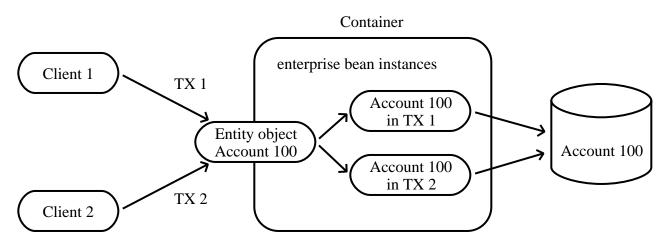
Figure 7. Multiple Clients Can Access the Same Entity Object Using Multiple Instances
