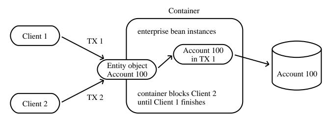
Figure 14. Multiple Clients Can Access the Same Entity Object Using Single Instance
