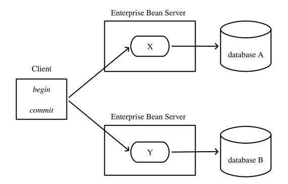
Figure 14. Updates on Multiple Databases on Multiple Servers
