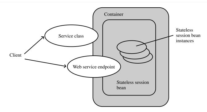
Figure 2. Web Service Client View of Stateless Session Beans Deployed in a Container
