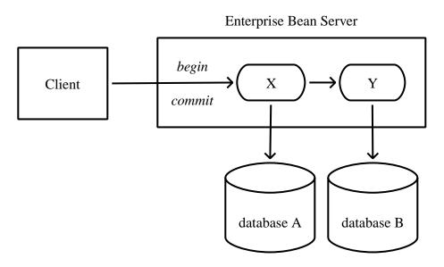
Figure 15. Update of Multiple Databases from Non-Transactional Client
