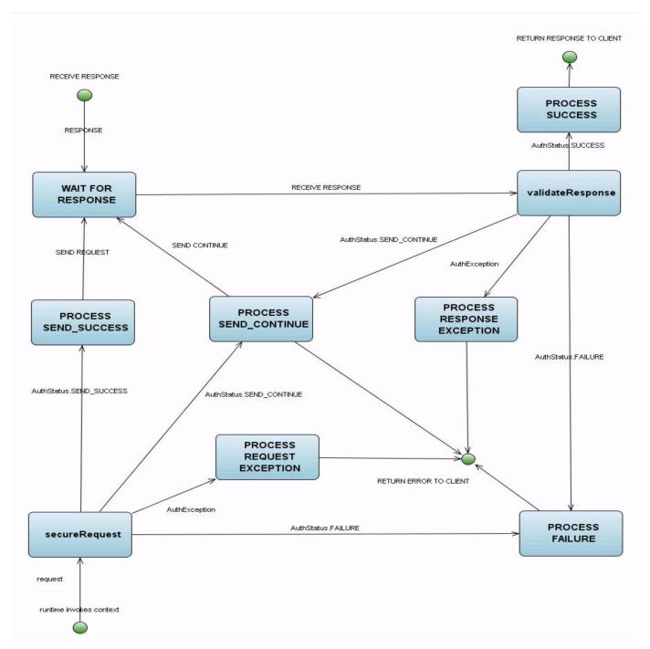
Figure 2-2 State Diagram of Client Message Processing Runtime
