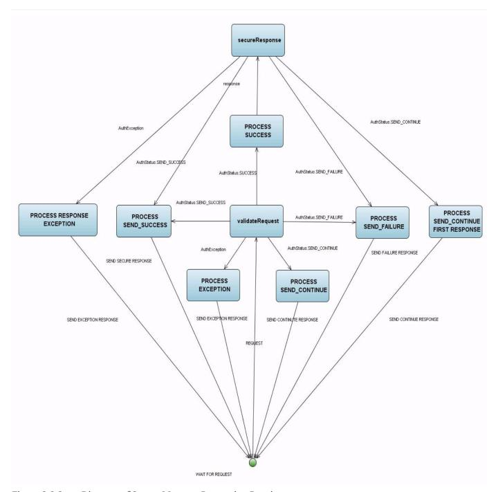
Figure 2-3 State Diagram of Server Message Processing Runtime
