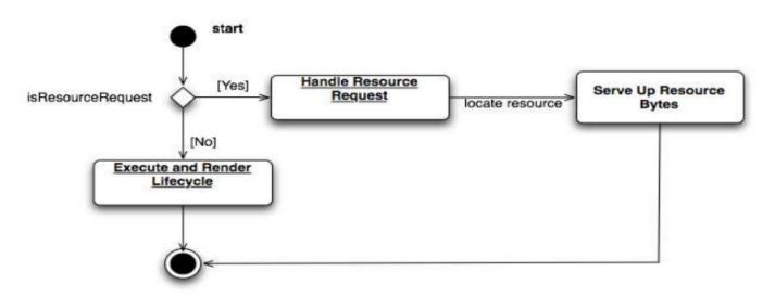
The "Handle Resource Request" box, and its subsequent boxes, are explained in Resource Handling. The following diagram explains the "Execute and Render Lifecycle" box.
